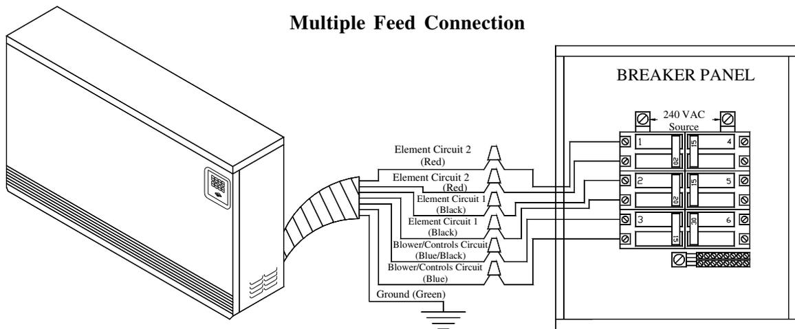
**NOTE:** Connections shown are for systems with a 240V/208V blower/controls circuit.
